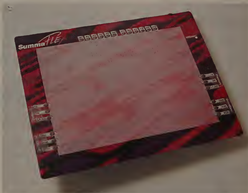
THE SUMMAFLEX can be rolled out onto any desktop and used as a drawing tablet and work surface.
